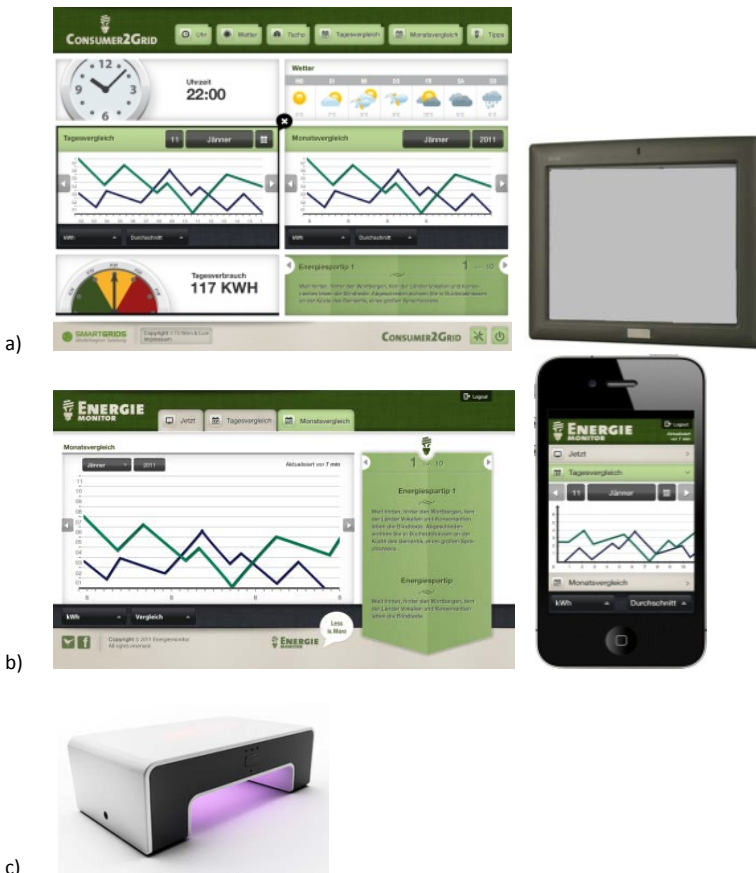
Figure 11. a) C2G home display, providing real-time feedback, detailed daily and monthly statistics, weather information, a clock and energy saving advices b) C2G web portal, accessible via PC and Smartphone, providing real-time feedback, monthly, detailed daily and monthly statistics and energy saving advices, c) Wattson [6], providing ambient real-time feedback via color coded light and/or consumption data
